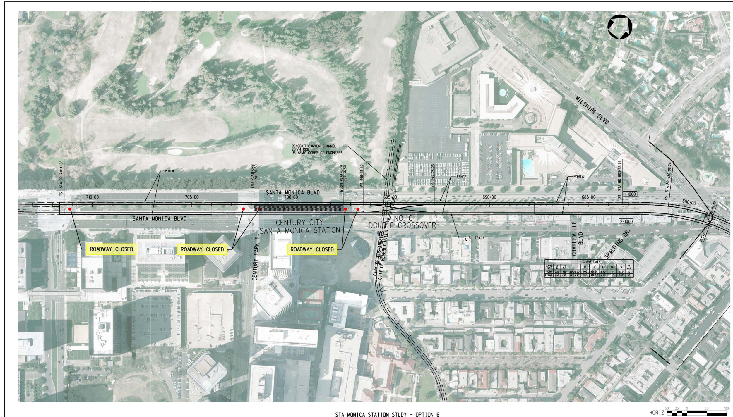
Figure A-15: Plan of At-Grade Station Concept
