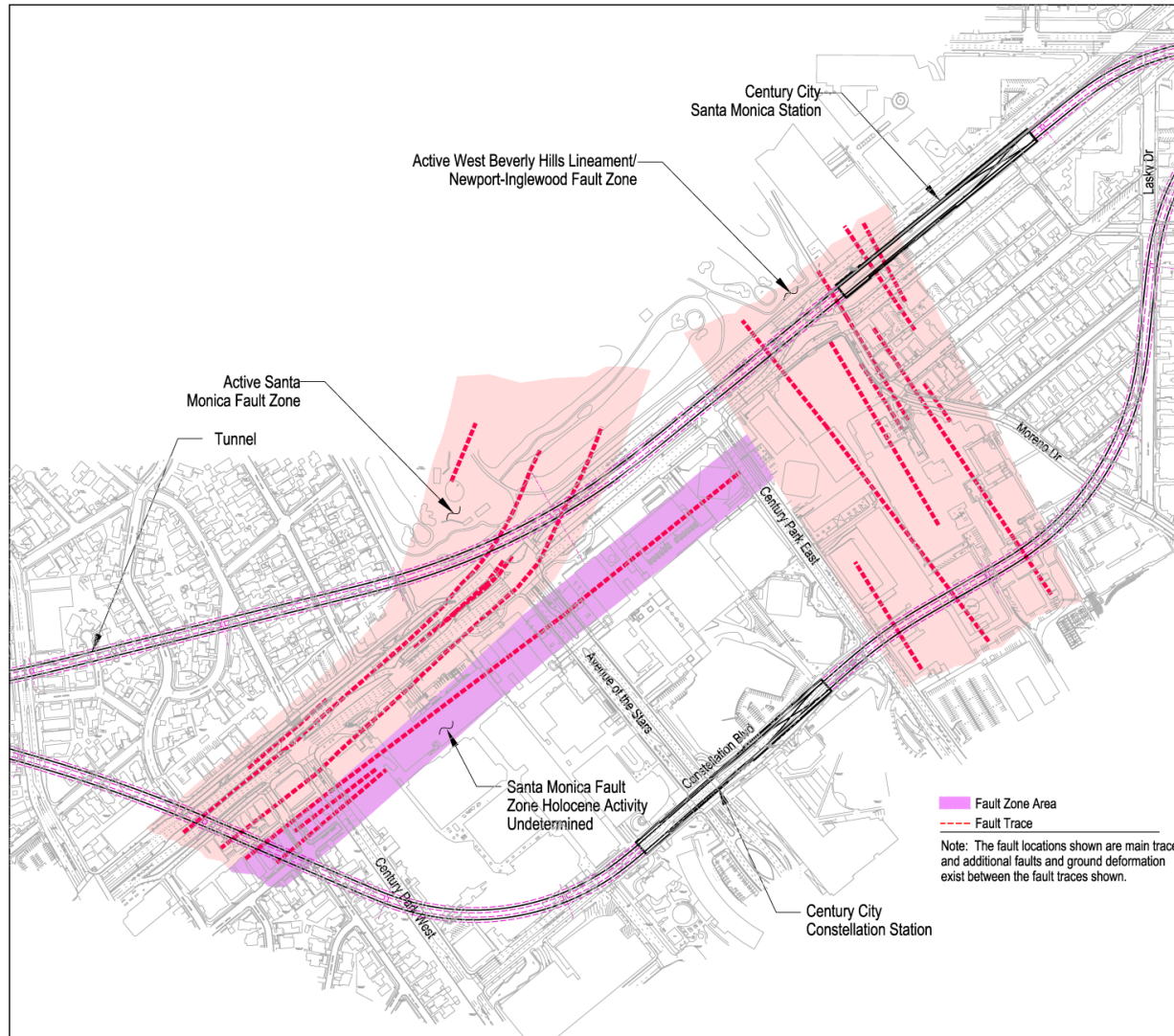
Figure A-14: Fault Zones, Century City, Santa Monica Boulevard Underground Station (Station East of Moreno Drive)
